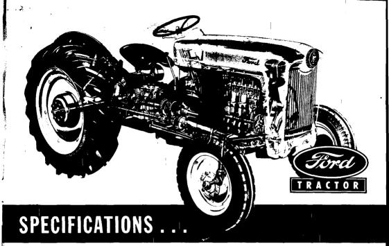
Regular Equipment: Rubber tires, safety starter, built-in hydraulic mechanism with Con-stant Draft and Implement Position Control and engine driven vane type pump, battery, genera-tor, voltage and current regulation, thermostat, oil pressure gauge, ammeter, temperature gauge, Proof-Meter, oil bath air cleaner, Full-Flow oil filter, adjustable wheel spacings, adjustable drawbar, drawbar stays and top link, fenders, muffler, tool box.
